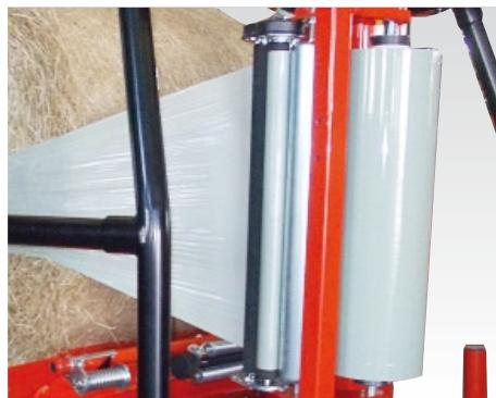
Distributore film di polietilene: pretensionamento standard al 55%. Polythene sheet distribution: standard pre-tension 55%. Distributeur de film polyéthylène: pretension standard 55%.
